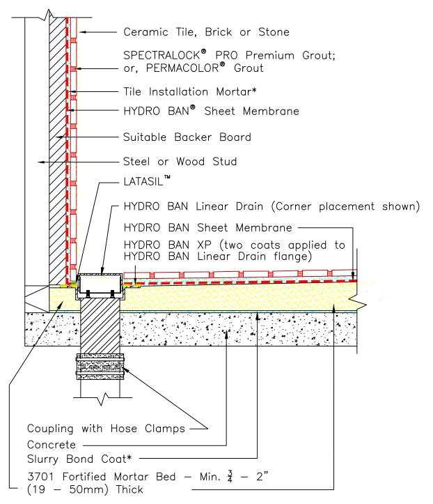
\* Slurry bond coat and tile installation mortar to be either 254 Platinum, 257 TITANIUM™ or MULTIMAX™ LITE.
